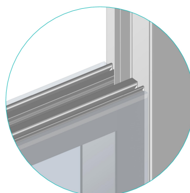
Connecting of the partition panel with the glazing
