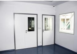
Basic partition panels represent one of the basic elements to construct clean workplaces and areas with maximum safety, sterility, hygiene, easy maintenance and sanitation.
