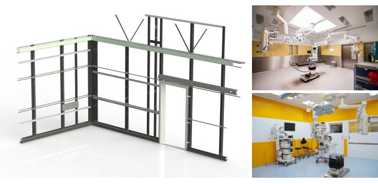
The Surgical bearing system ensures even distribution of load from individual components to supporting structures. The whole system is designed so that it allows the creation of all the necessary structural details necessary to build operating theatres and adjoining facilities. The system is built of galvanized steel metal sheet. Individual components are bolted to each other and the entire system is connected to the grounding of the whole structure.
