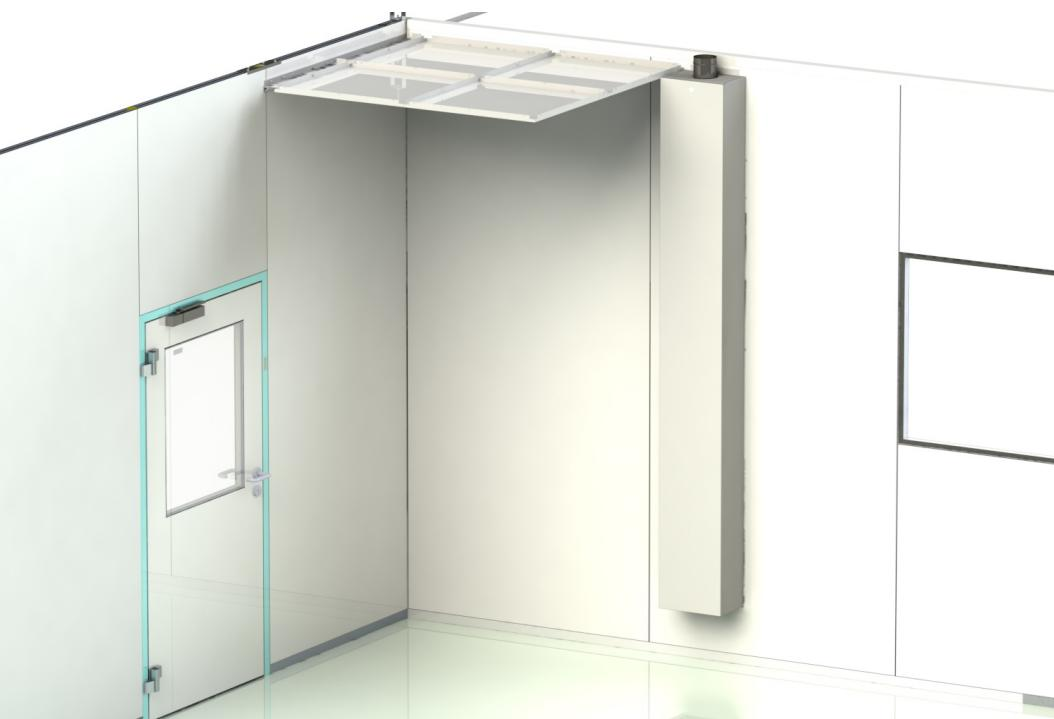
The air duct is used to remove air from clean rooms in the system of sandwich partitions. This air duct is suspended (it is anchored to the partition panel) and is not part of the partitions (it protrudes into the room space).
