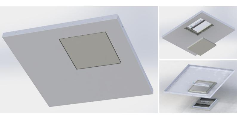
A smoke exhaust panel for ceiling. The panel is designed as a gravitational system for the exhaust of heat and smoke in the case of an emergency - fire. Suitable for operating rooms, preparation rooms, clean laboratories and clean warehouses. The panel is integrated in a walkable suspended ceiling panels of 1170x1170 mm, 625x625 mm. The panel is used as a safety device.
