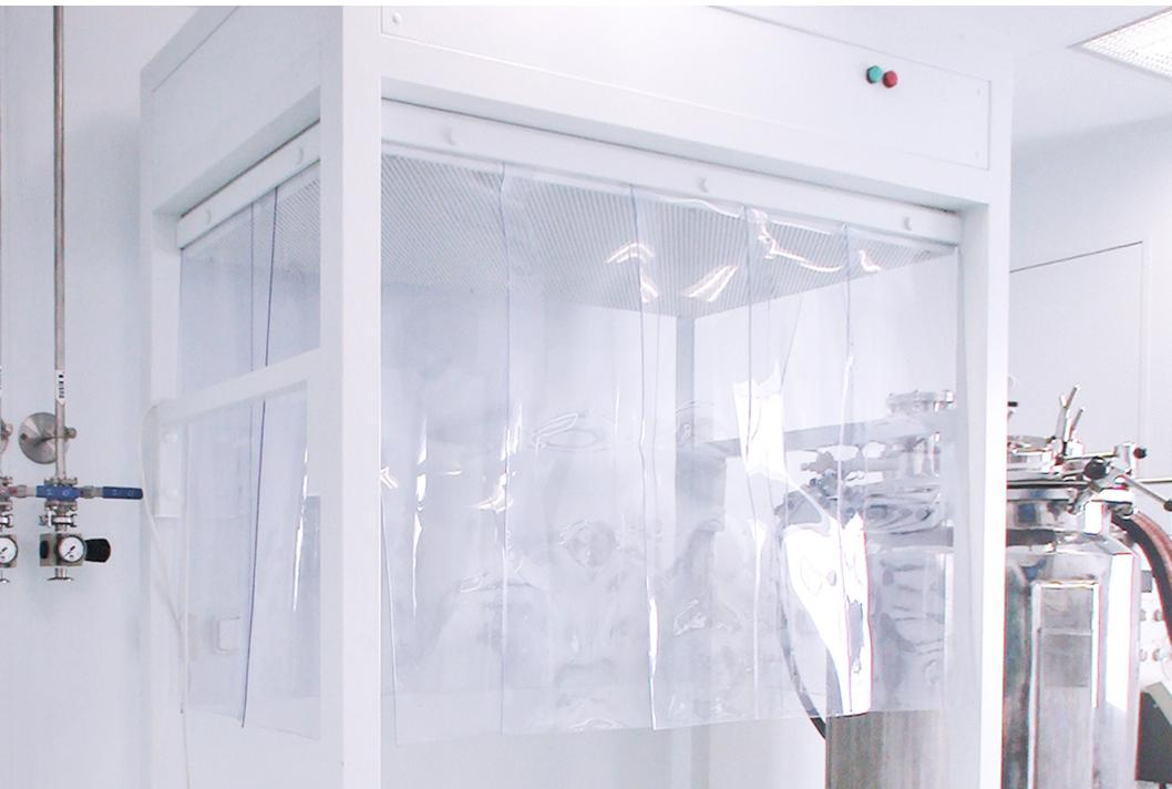
The movable box is a corpus for mobile device equipped with circulating units, which is used (together with flexible screens, which increase the protection of the product) to set up a closed workplace with uniform airflow, lighting and the required class of cleanliness.
