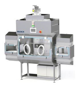
Isolator provides a high degree of protection for the personnel working with cytostatic and otherwise hazardous materials. It works in a negative pressure atmosphere in cleanliness class "A", with a laminar airflow of 0.45 m/s  $\pm 20\%$ . Isolator can be used for example, in pharmacies or hospitals, for preparation (dilution and dosing) of cytostatic and followed by drug administration to patients.
