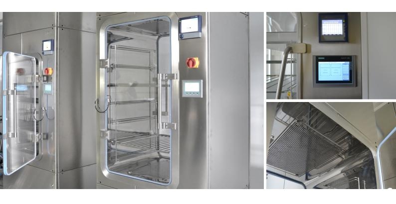
Decontamination pass-through cabin is most frequently used as material pass-through to transfer material between rooms with different classes of cleanliness (typically B and C). Equipment and materials are decontaminated in a decontamination cycle using hydrogen peroxide vapour. Hydrogen peroxide vapour generator is part of the pass-through decontamination cabin; the two form a single piece of equipment.
