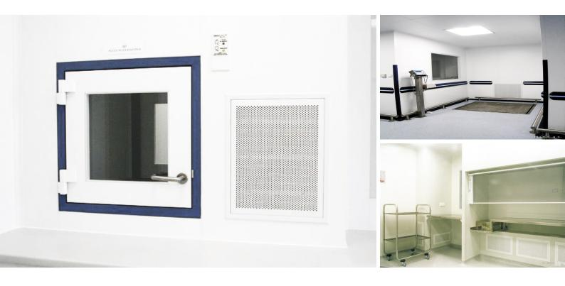
Air conditioning grilles are used to exhaust air from clean areas. They are the end exhaust element with a direct connection to the HVAC exhaust pipeline, exhaust ducts, they can be installed in metal panels (even double-sided version), plasterboard partitions, doors of exhausted cabinets, etc.
