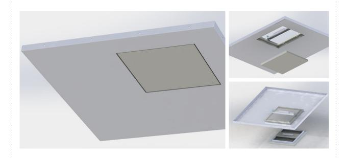
A smoke exhaust panel for walkable suspended ceiling. The panel is designed as a gravitational system for the exhaust of heat and smoke in the case of an emergency - fire. Suitable for operating rooms, preparation rooms, clean laboratories and clean warehouses. The panel is integrated in a walkable suspended ceiling panel of 1170x1170 mm. The panel is used as a safety device.
