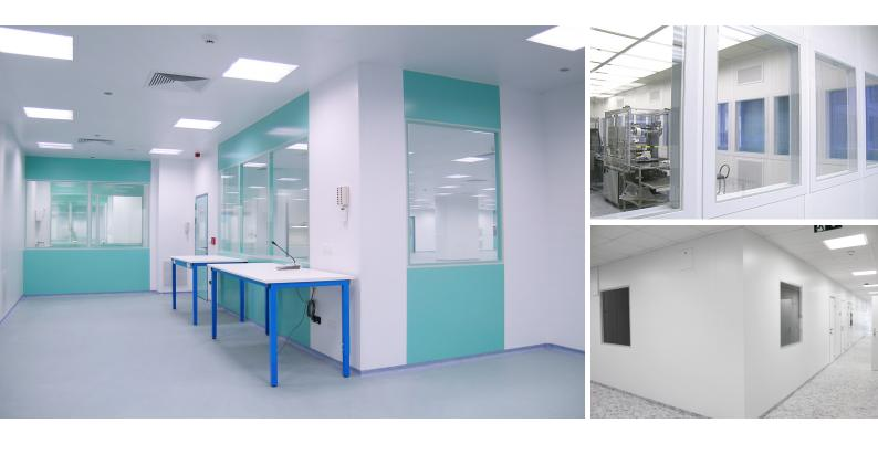
With the system of partition panels, a glazed window panel represents one of the basic elements to construct clean workplaces and areas with maximum safety, sterility, hygiene, easy maintenance and sanitation.
