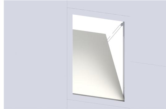
Door for air inlet for partition systems of 60 mm thickness.
